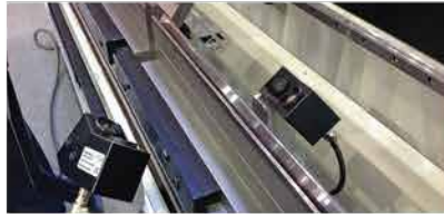
Sensor laser para lectura del ángulo del pliegue. Laser based device for measuring bending angles.
